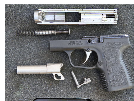
The Kahr CM9 field strip for routine cleaning
